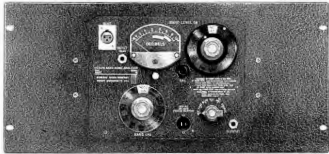
Relay-rack model, Type 1558-9820 (or Type 1558-9822), is adapted from portable model; see page 210.
